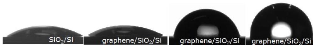
Figure A4.10. Irreproducibility of the WCA of graphene transferred onto SiO 2 /Si wafers: WCA of bare SiO 2 /Si wafer and WCA of graphene transferred onto SiO 2 /Si wafer for different samples.
