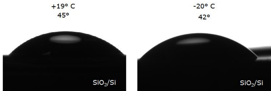
Figure A4.3. Control water contact angle on SiO 2 /Si under ambient conditions (left) and under conditions identical to the measurements with ice (right). For the latter the wafer was placed on the surface of water solution of ammonium persulfate and then cooled down to -20°C in Peltier chamber with constant flushing the chamber with dry air. No significant difference in WCA was detected
