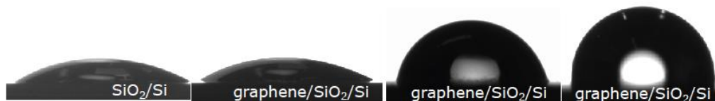
Figure A4.10. Irreproducibility of the WCA of graphene transferred onto \text{SiO}_2/\text{Si} wafers: WCA of bare \text{SiO}_2/\text{Si} wafer and WCA of graphene transferred onto \text{SiO}_2/\text{Si} wafer for different samples.
