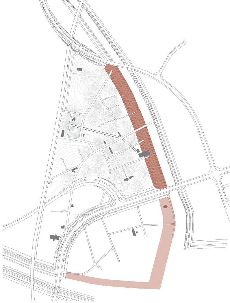
Under the current masterplan proposal, the southern portion of the park is enclosed by two seawalls. By removing the redundant seawall, we have the opportunity to create an area of the park which would be open to the influences of the ocean. This environment would be a rich habitat for salt marsh flora and fauna, as well as a site for clam collecting activities attractive to both locals and visitors.
