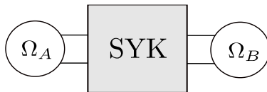
Figure 6.1. Cheburashkian geometry [135]. Two quantum dots with discrete energy levels \Omega_A and \Omega_B are symmetrically coupled to an SYK quantum dot.
