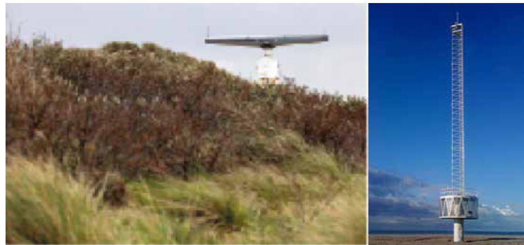
Figure 2. X-band radar station (left) and Argus video tower (right) at the Sand Motor.
