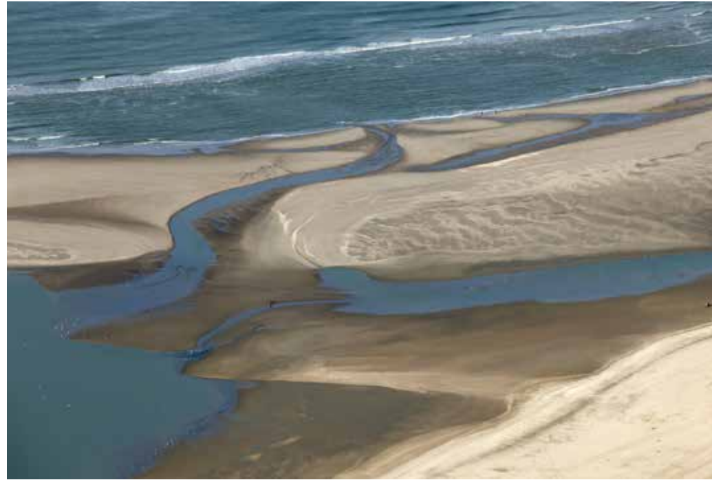
Figure 3. The Sand Motor lagoon is a shallow artificial area that was created to serve as a nursery for juvenile fish, offering shelter and increased temperatures. Over time the entrance channel to the lagoon has reduced in depth and width. (Photo by Rijkswaterstaat/Jurriaan Brobbel)
