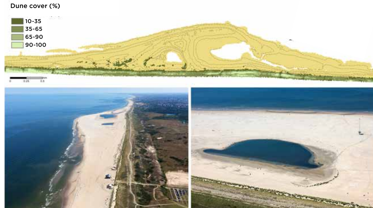
Figure 2. The state of dune development on and along the Sand Motor in the summer of 2017. (Data derived from satellite imagery, photos courtesy of Rijkswaterstaat and Jurriaan Brobbel.)
