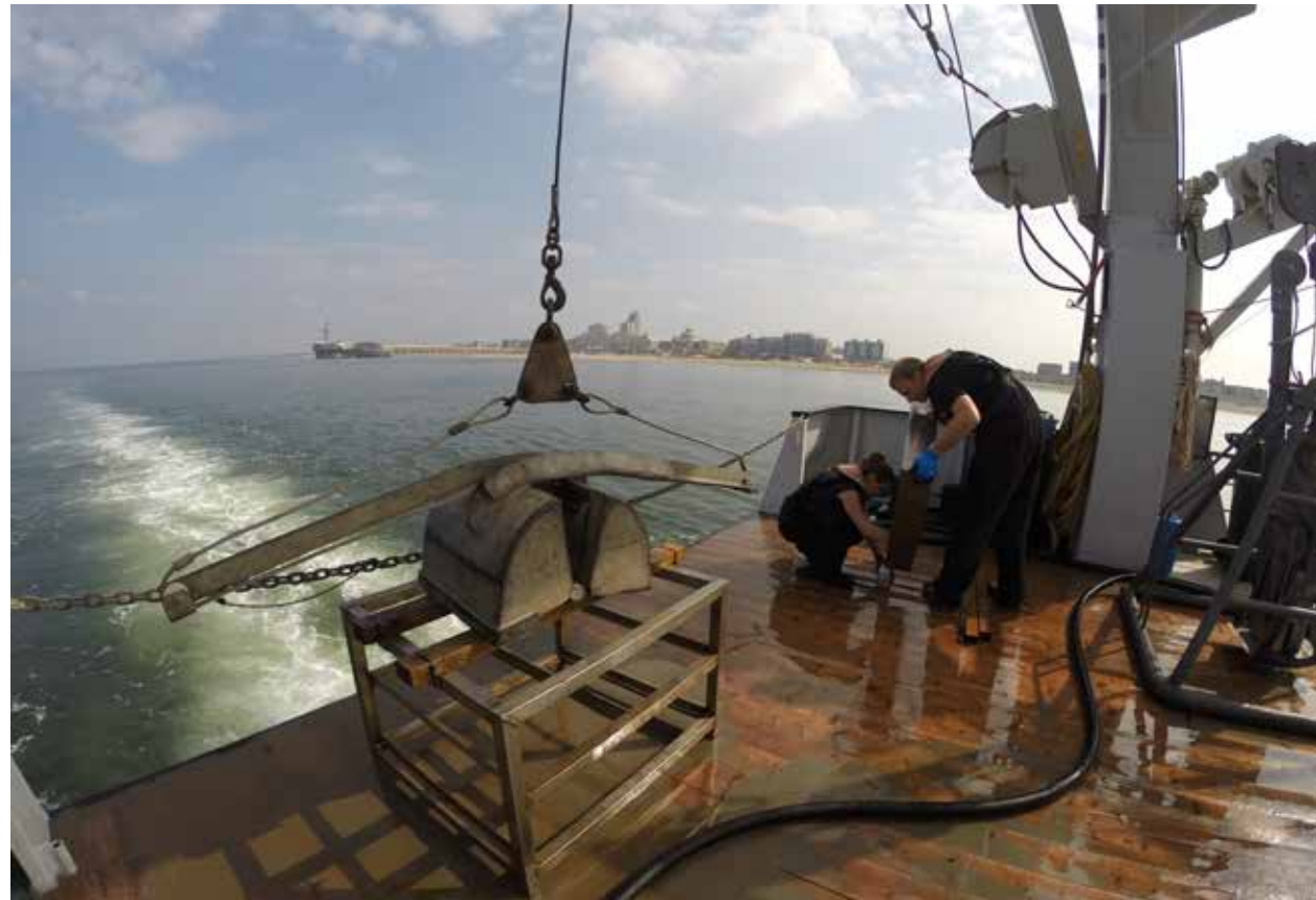
Figure 2. A sample is taken from the seafloor with a "Van Veen Grab Sampler" near the coast at Scheveningen, the Netherlands.
