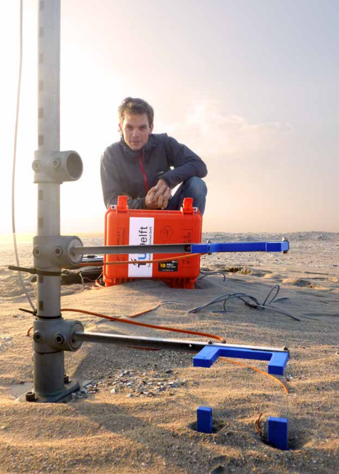
Figure 2. (left) Measurement equipment with laser sensors deployed at the Sand Motor.
