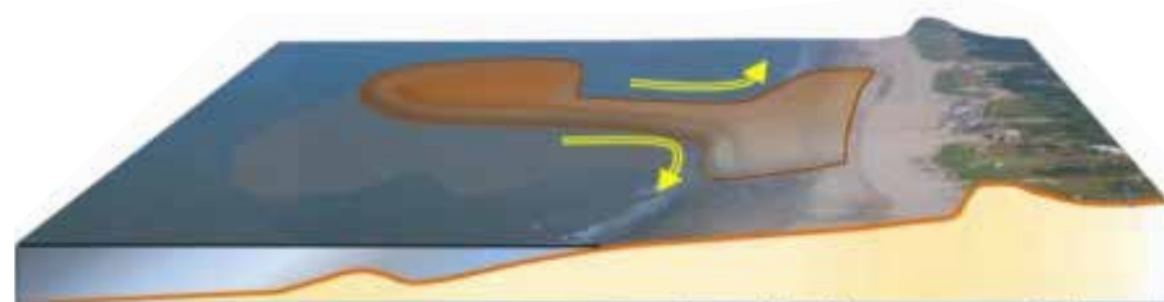
c Localized mega nourishment
