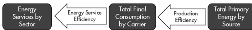
Figure 4.1 – Primary energy metrics and efficiency indicators. Energy services by sector need to be supplied by energy carriers which need to be produced from energy sources.
