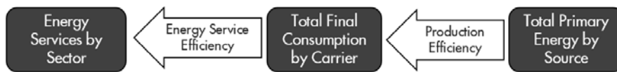
Figure 4.1 – Primary energy metrics and efficiency indicators. Energy services by sector need to be supplied by energy carriers which need to be produced from energy sources.
