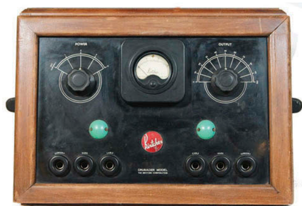
Figure 5. The Birtcher Crusader developed in the 1930s, a forerunner of the Hyfrecator (From the collection of John Abele, with kind permission of John Abele and Steven Schwaitzberg).
