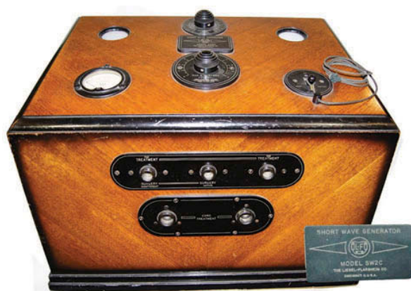
Figure 4. Liebel-Flarsheim short wave radiofrequency generator from the 1930s (From the collection of John Abele with kind permission of John Abele and Steven D. Schwaitzberg).
