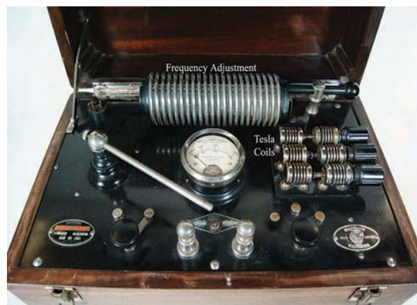
Figure 2. McIntosh diathermy with adjustable frequency and Tesla coils (From the collection of John Abele with kind permission of John Abele and Steven D. Schweitzberg).
