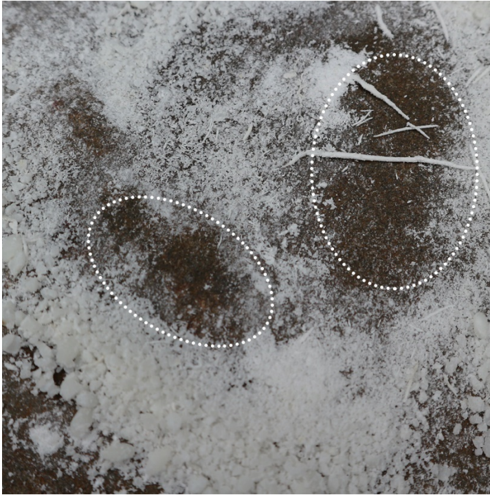
Figure 3.3 Soaked rice flour forms the “noodle shapes” during wet-grinding (the ellipse illustrates the exposed stone surface).
