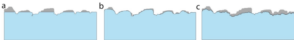
Figure 4: Illustrations of micro-polish with (a) flat, (b) domed and sinuous, and (c) irregular topography (After Wang, 2019)
