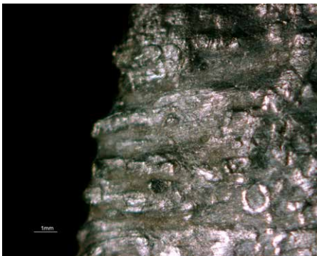
Fig. 5.21 Experimentally using a battle axe to uproot a tree; (bottom) pictures taken with stereo microscope of the cutting edge showing extensive edge damage and ca. 1 mm wide striations are clearly visible.
