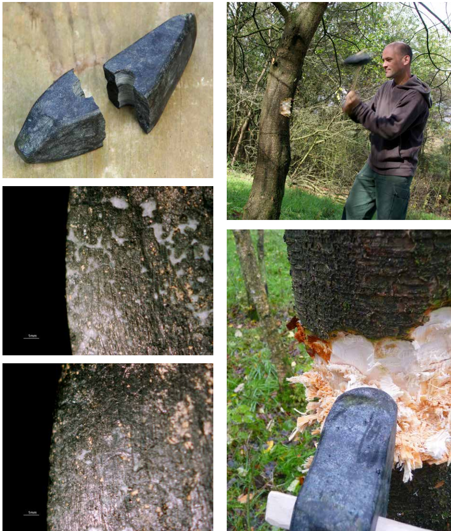
Fig. 5.20 Experimentally using a battle axe to chop a tree; (top right) broken battle axe (after 5 minutes of use); (centre and bottom right) pictures taken with stereo microscope of cutting edge of second battle axe, some rounding and minor edge damage can be seen, shallow scratches are part of production traces (grinding).
