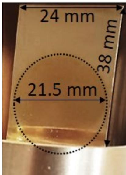
Figure 2.9: The darker circle, outlined by a dashed circle, is carbon deposit that resulted from the atomic beam on the gold surface of the substrate. The entire beam is on the flat surface, and the angle at which the picture is taken makes it appear that the lower part is clipped. A beam diameter of 21.5 mm is measured on a sample plate that has a size of 38 mm  $\times$  24 mm. Note that contrast has been added to the image to visualize the area with impacting C-atoms.
