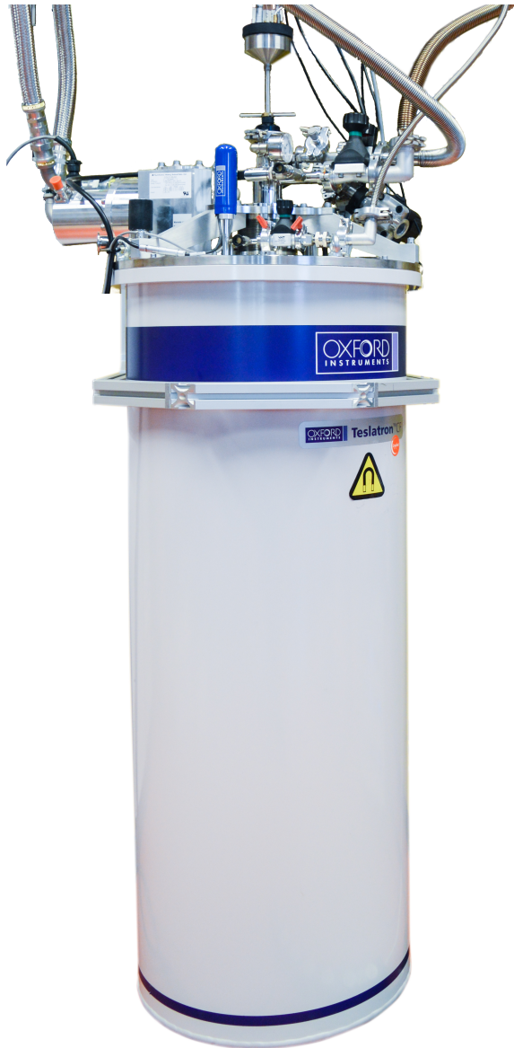
Fig. 4.1: Picture of the cryostat as installed. The rotary valve feeding the pulse tube can be seen on the top left, connected to two (one supply, one return) high pressure helium lines. The various lines in the top right are from right: insert vacuum line, helium circulation return (big line), helium circulation supply (small line).
