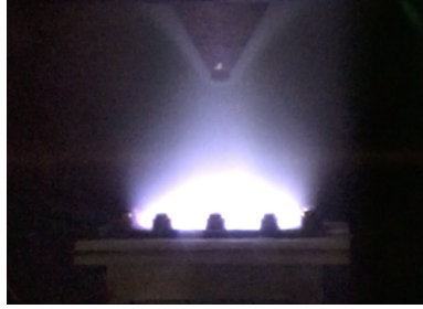
Figure 1.7: A typical acetylene plasma expansion produced from the SPIRAS slit discharge nozzle.
