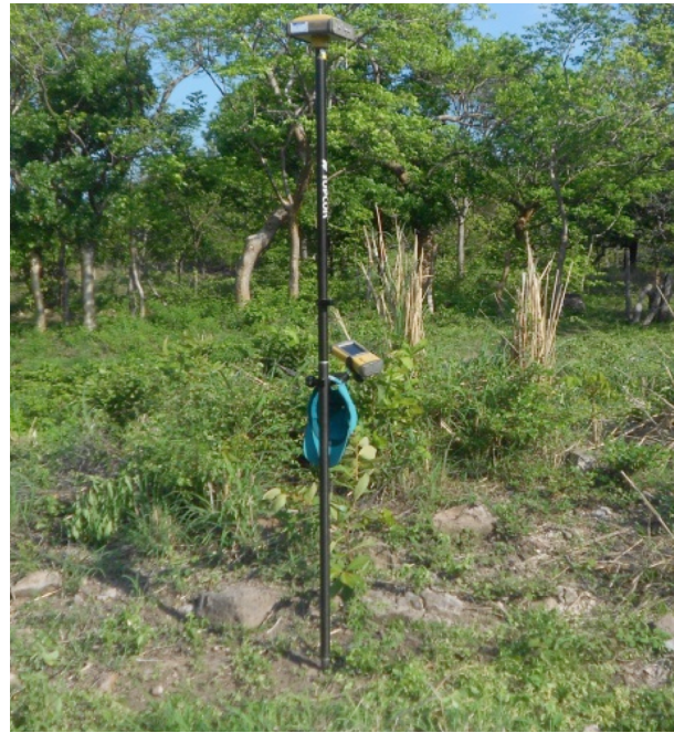
Figure 2b: A differential GPS Rover.
