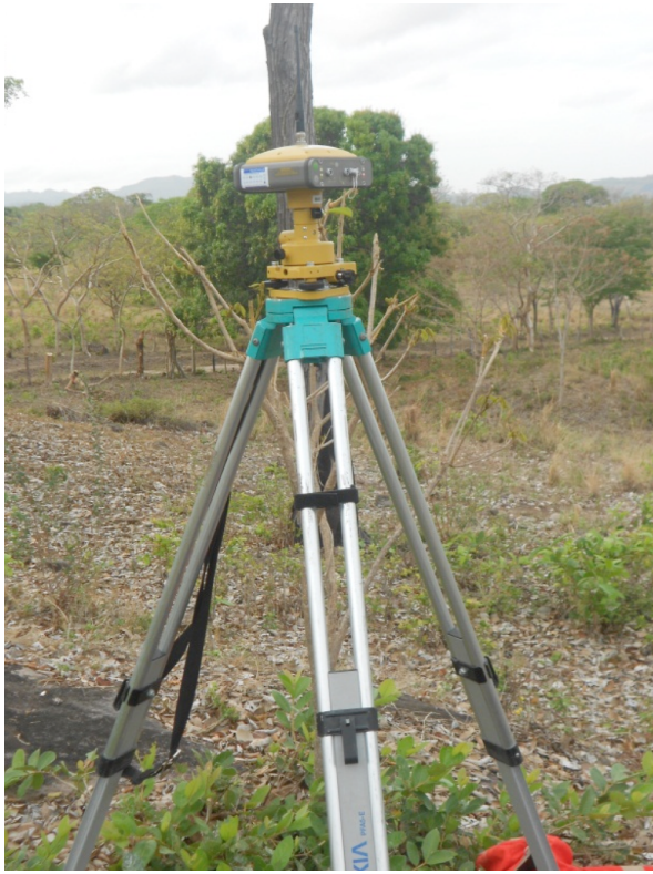
Figure 2a: A differential GPS Base Station .
