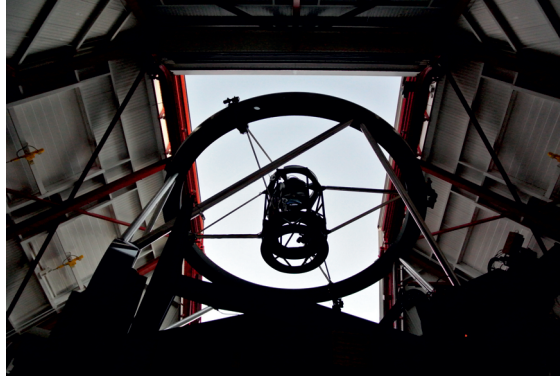
Figure 1.6: Secondary mirror (M2) of Magellan’s Clay telescope. The secondary is the deformable mirror for the Magellan adaptive optics system MagAO.
