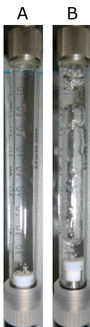
Figure 3: Fig. 3. Image of the PAMAS SBSS light obscuration syringe pump aspirating A) purified water and B) 75% (w/v) sucrose solution during sample measurement at ambient pressure conditions.
