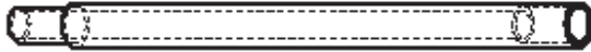
Figure 2.2: Illustration of piece of PEI. The total length is 30 mm and has an outside and inside diameter of 2 and 1 mm, respectively.
