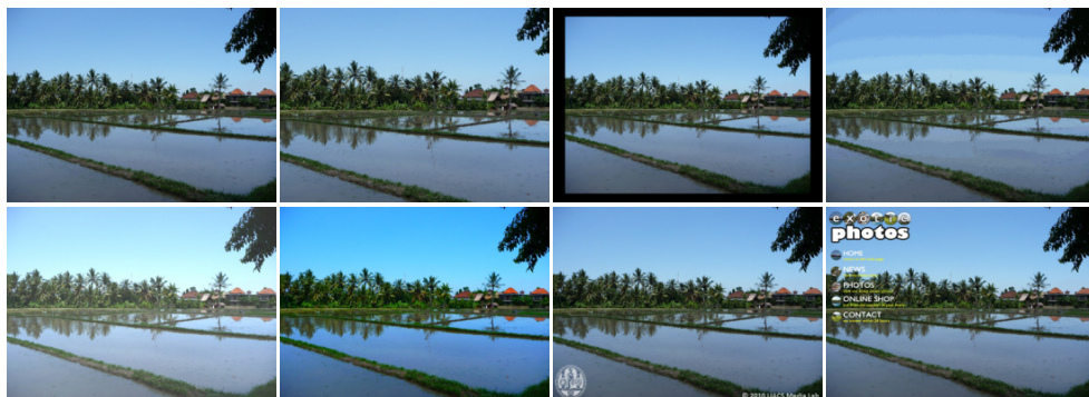
Figure 6.10: Examples of image transformations. Clockwise, starting from the top-left: original image, crop, letterbox, convert to 256 colors, menu, copyright, increase in saturation, increase in intensity.
