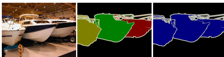
Figure 1.7: Example image from the Pascal VOC collection containing boats (left), the segmentation into individual objects (middle) and classification into the boat category (right).
