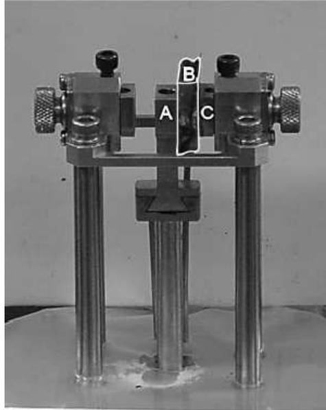
**Figure 4.2:** Experimental set-up of the Dynamic Mechanical Analyzer (DMA). One shaft (A) moves and the other shaft (C) does not move, so a sinusoidal strain is generated to the thrombus samples (B).
