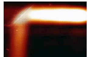
Figure 1: A Flatland mirror, seen from above; it is tilted at 45°. The surface plasmon enters from the right side of the figure and is partially reflected downwards. (Reprinted from González et al. (2006), with kind permission of the author. Copyright 2006, the American Physical Society.)
