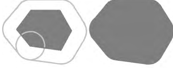
Figure 3.8: Example of a dilation process of an anchor region by a circular structuring element. Dark area to the left is the anchor region being dilated, resulting in the dark area to the right.
