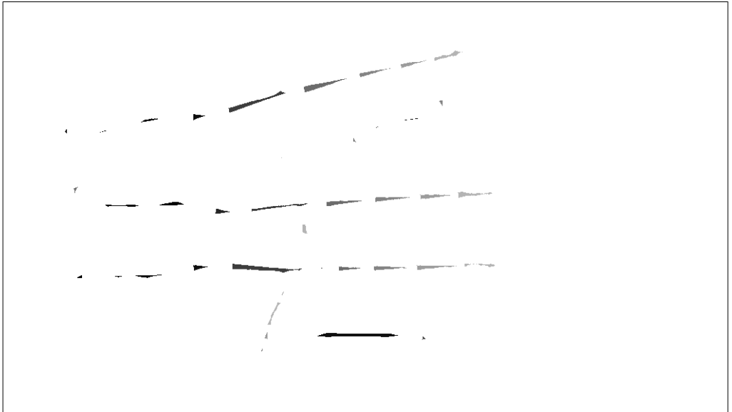
Figure 3.7: D_{best} : a collection of anchor regions a_0, \dots, a_n selected from the Distance Transform of example in Figure 3.3. d for each a is encoded as a grayscale value. Image saturation contrast has been improved for visual purposes.
