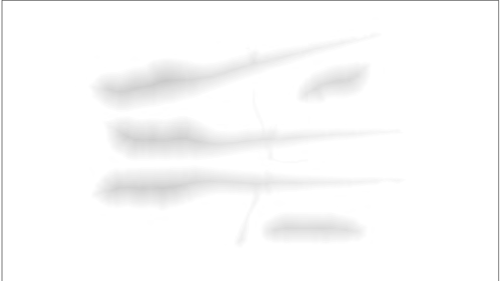
Figure 3.6: Euclidean Distance transform D of the binary image from Figure 3.3. An inverted lookup table is used, therefore the lighter pixels correspond to low DT function values (closer to the background) and dark pixels correspond to high values (further from the background).
