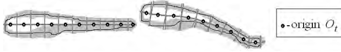
Figure 2.19: A prototype template as a chain of slices and a deformed instance. All shape boundaries that fit in the grey area fit the template. Black lines represent two example shapes that fit these templates.
