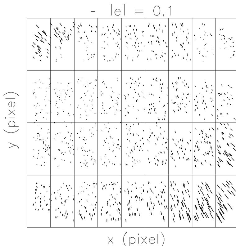
**Figure 1.13** Point-spread function (PSF) pattern of a typical field in the Canada-France-Hawaii Telescope Legacy Survey (CFHTLS). Each tick represents the observed magnitude and orientation of a stellar ellipticity. The artificially induced ellipticity is most prominent in the corners in this case. Figure originally published in Fu et al. (2008).
