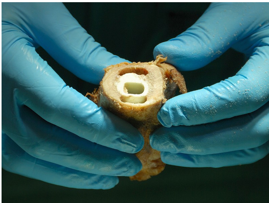
Figure 2.4 – Femoral lesions mechanically created anterior and posterior of the cement mantle are shown with the prosthesis removed.
