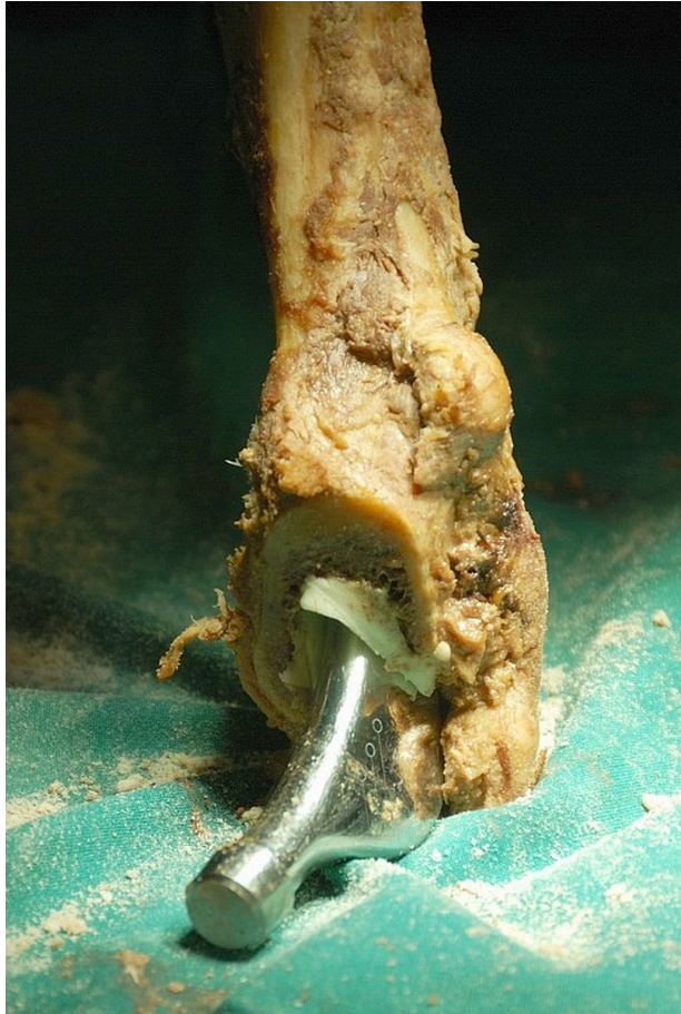
Figure 2.3 – The removable Exeter prosthesis is shown partly dislodged from one of the test femora.
