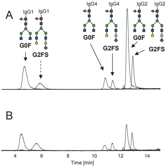
**Figure 2.** Comparison of the different sprayers for IgG Fc N-glycopeptide ionization. Extracted ion chromatograms obtained with a metal nano-ESI sprayer (A) and a sheath-flow ESI sprayer (B). Figures are represented with the same scaling. IgG Fc N-glycopeptides were separated at 500 nl/min using an ACN gradient with FA as mobile phase additive. The sheath-flow sprayer was applied with a 2  $\mu$ l/min sheath-flow of 50% IPA containing 2% PA. Glycan code as in Figure 1 of Chapter 1.
