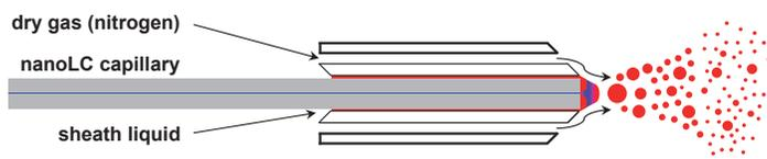
**Figure 1.** Schematic representation of the sheath-flow ESI sprayer.
