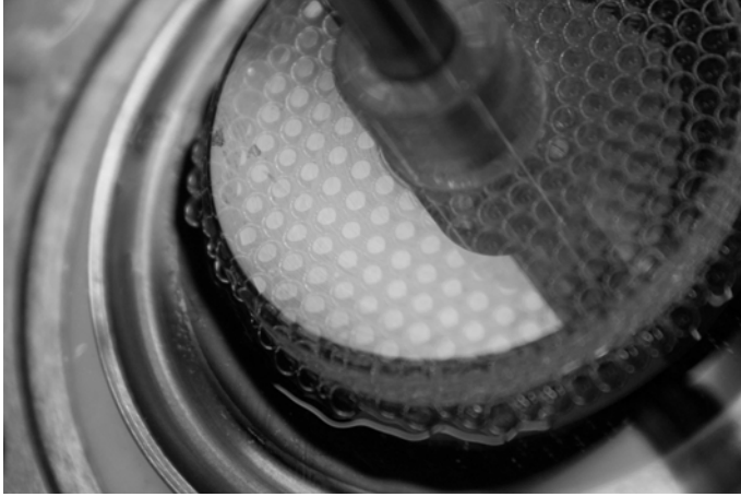
FIGURE 2.10: Close-up photograph of the rheometrical tool used to measure the bubble-wall drag. The radius r_c is clearly visible in reflected light and is used to extract R_0 .
