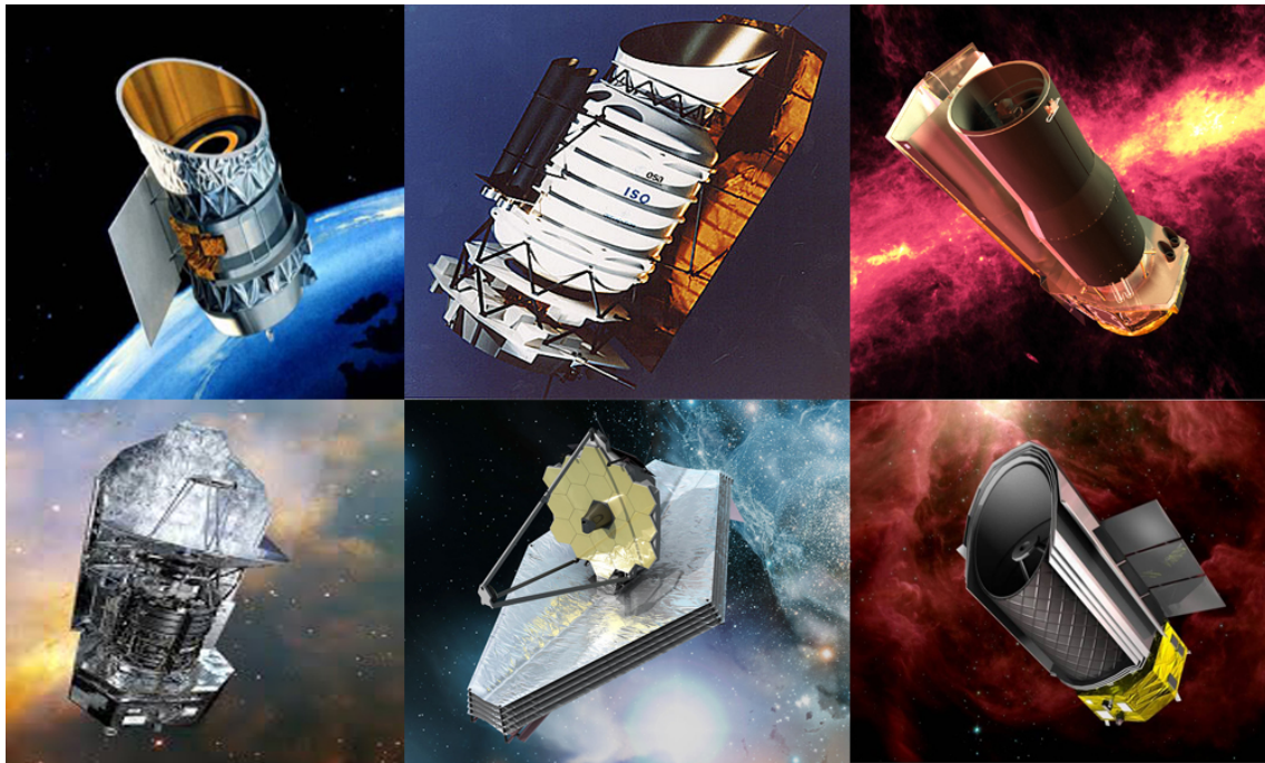
Figure 1.5: Six generations of space based infrared telescopes. New telescopes often improve spatial resolution, spectral resolution and sensitivity. Top, from left to right: the Infrared Astronomical Satellite (IRAS) launched in 1983, the Infrared Space Observatory (ISO) launched in 1995 and the Spitzer Space Observatory launched in 2003. Bottom, from left to right: the Herschel space telescope launched in 2009, and the James Webb Space Telescope (JWST), with a proposed launch in 2018 and the Space Infrared Telescope for Cosmology and Astrophysics (SPICA), with a proposed launch in 2025.
