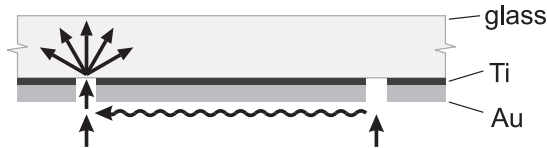
Figure 2.2. Two interfering paths leading to light emission from the leftmost slit. A similar set of paths gives rise to emission from the slit on the right-hand side. The dashed line indicates the propagating surface plasmon.
