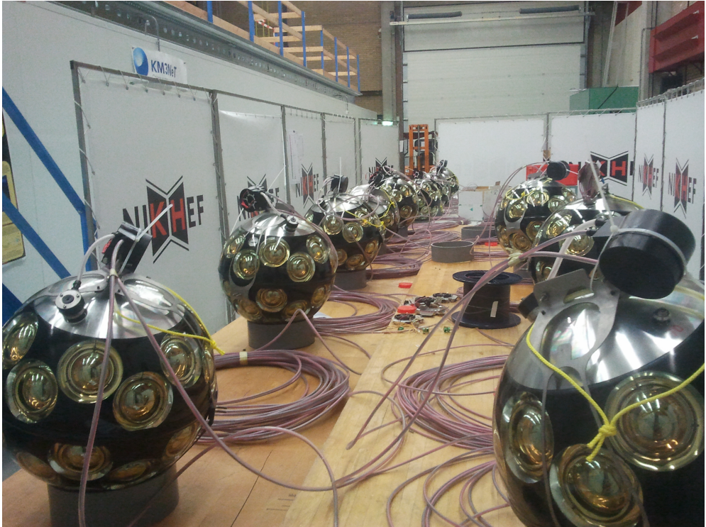
Figure 6.2: Photo of the recently completed KM3NeT string. The Multi-PMT optical modules can also be seen.
