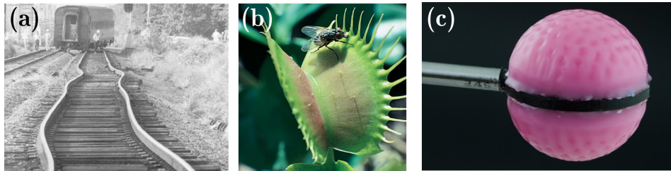
FIGURE 1.5: (a) Buckling as failure, sun kinks in railroad tracks. Image courtesy of AP (b) The rapid closing of the mouth of a venus fly trap is induced by a snap-buckling instability. Image courtesy of www.carolina.com (c) Wrinkling patterns at the surface activated by elastic instabilities. Image courtesy of MIT/P.Reis
