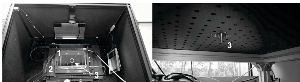
Figure 8.19. Photographs of setup used for irradiation experiments with high intensity red light, consisting of a mini-incubator (1; for clarity here without 96-well plate), motorized XY-translation stage (2), and collimating lens fitted underneath the mini-incubator (3), connected to a fiber-coupled laser (not shown).
