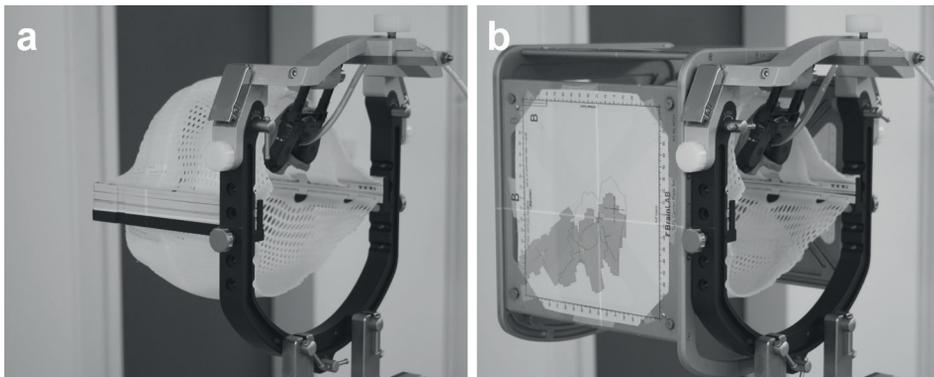
Figure 5. BrainLAB Mask System with VMP. Overview of the complete setup. (a) Without the Target Positioner Box. (b) With the Target Positioner Box.
