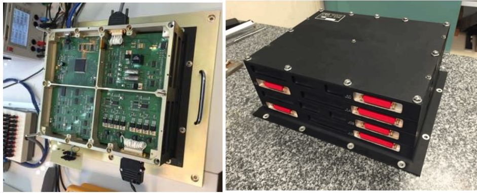
Figure 10: Two views of the EM PMCU which controls the shutter, calibration unit and provides the thermal control of the FPA.
