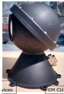
Figure 8: The EM Calibration Unit. This unit lacks the baffle on the exit port (on the left) with its field stop and lens system.
