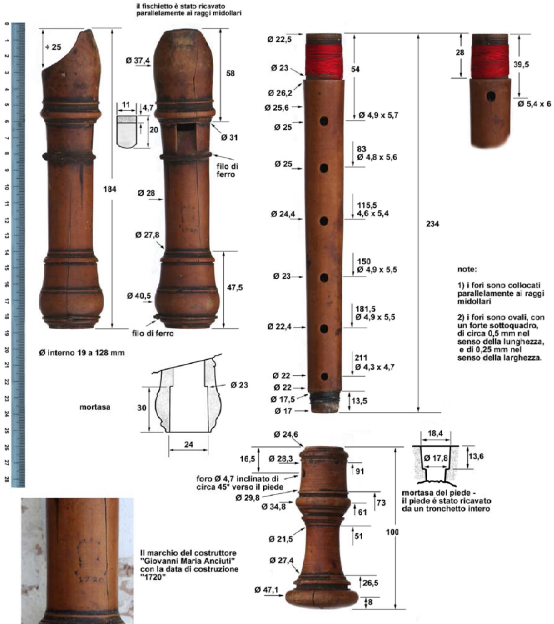
Figure 16. Drawings and measurements of the 1720 Anciuti alto, extracted from the plan by R. Gandolfi and V. Biella ( http://www.baghet.it/Flauto%20di%20Montoggio.pdf ).
