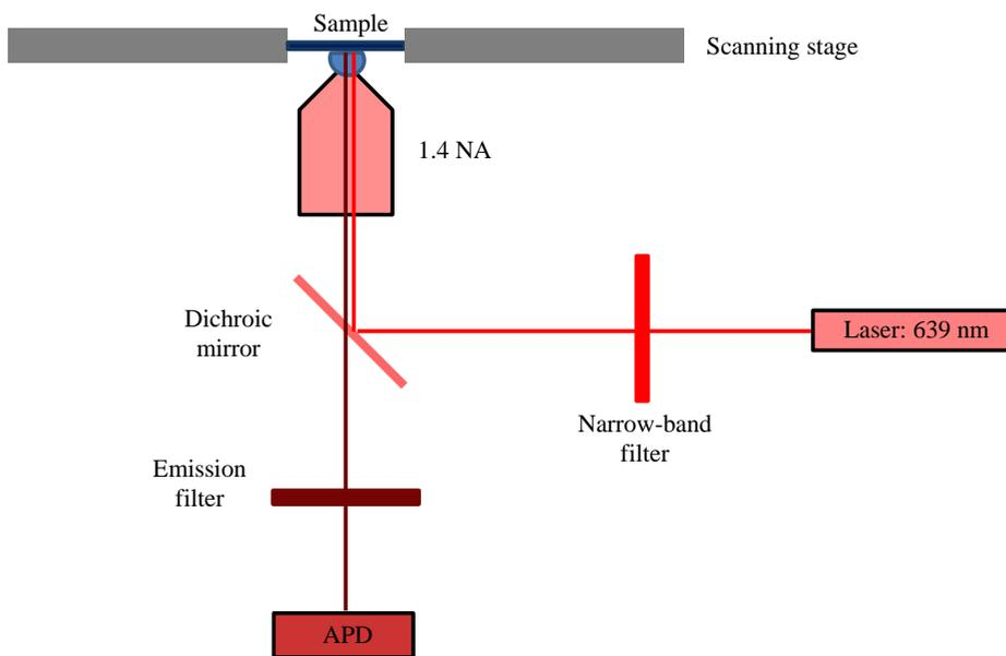
**Figure 1.5:** Setup for time-resolved measurements. A pulsed laser light ( $\lambda = 639$  nm) is filtered through the narrow-band filter and reflected by the dichroic mirror through the oil-immersion objective onto the sample mounted on the scanning stage. The emitted light is collected by the objective and transmitted through the dichroic mirror and emission filter to a single-photon counter (APD).
