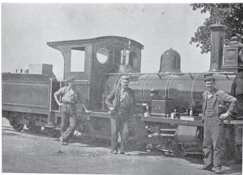
Fig. 6.5 Beira Railway Falcon 4-4-0 no. 24 with six-wheel tender after repaint (many white enginemen on the railways took great care in looking after 'their' engines) (Source: A.H. Croxton, Railways of Rhodesia , David & Charles Publisher, 1973, p. 66)
