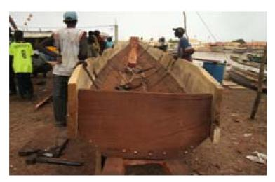
Construction of a Piroque
