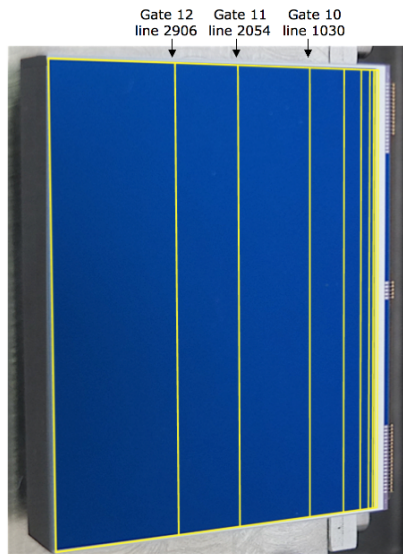
Fig. 2. Gaia CCD with the position of the special TDI gates overlaid in yellow. The charge injection structure is to the left and the serial register to the right. Only the three TDI gates closest to the charge injection structure are marked. Towards the serial register the spacing between gates is successively reduced by a factor of 2 and becomes too closely spaced for illustration. The image orientation follows the Gaia convention with the scan direction in the image area from left to right. The physical dimensions of each device are approximately 4.7 \times 6.0 cm (AL \times AC).
