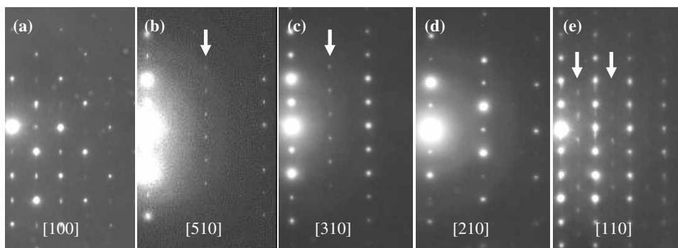
Figure 2. Electron diffraction patterns of the 3 nm LCMO ultrathin film (obtained by tilting the sample along the  $[001]_{\text{STO}}$  axis) which has been indexed as a simple-cubic structure. Note the presence of super-reflections as marked by arrows in (b), (c) and (e).
