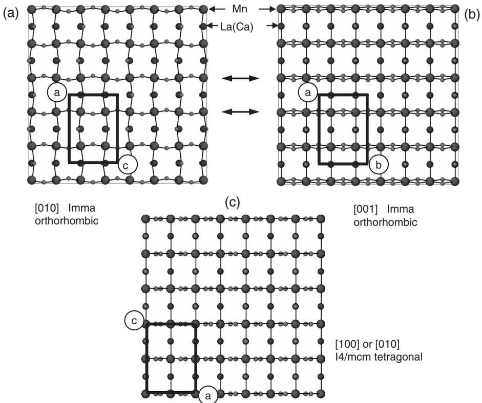
Figure 5. Comparison of proposed structures of  $(La,Ca)MnO_3$  based on two space groups. (a)  $[010]_{Imma}$  orthorhombic and (b)  $[001]_{Imma}$  zone view of the orthorhombic structure ( $Imma$ ), and (c)  $[100]_{I4/mcm}$  or  $[010]_{I4/mcm}$  zone view of the tetragonal structure ( $I4/mcm$ ). The unit cells are outlined by solid rectangles.
