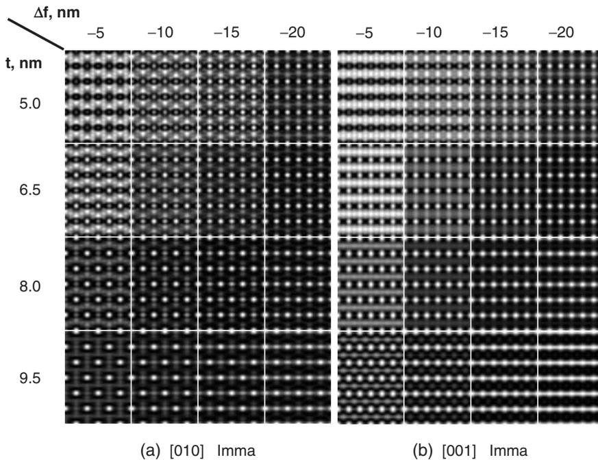
Figure 6. Matrix of simulated images of the orthorhombic structure  $Imma$  along  $[010]$  (a) and  $[001]$  (b) zones. The specimen thickness was varied from 5.0 to 9.5 nm and the defocus was varied over the range of  $-5$  to  $-20$  nm in steps of  $-5$  nm.
