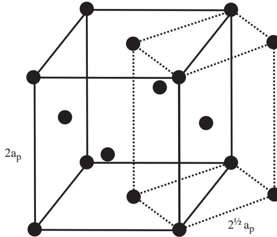
Figure 3. A schematic of the relationship between a face-centred cubic  $2a_p \times 2a_p \times 2a_p$  cell (outlined by the solid line) and a body-centred tetragonal or orthorhombic  $2^{1/2}a_p \times 2^{1/2}a_p \times 2a_p$  cell (outlined by the dashed line).
