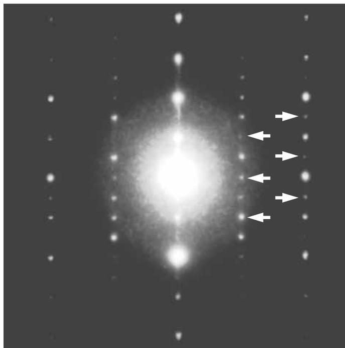
Figure 7. Electron diffraction pattern of a 5 nm LCMO film along [310]<sub>STO</sub> direction. Compared with figure 2(c) extra super-reflections present as marked by arrows, which indicate that it be indexed as the [201]<sub>Pnma</sub> zone pattern of the *Pnma* structure.
