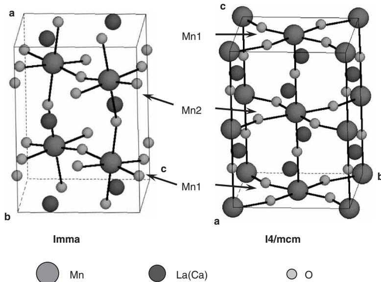
Figure 4. Comparison of proposed unit cell of (La,Ca)MnO<sub>3</sub> based on two space groups *Imma* and *I4/mcm*. The MnO<sub>2</sub> layers are marked by arrows.
