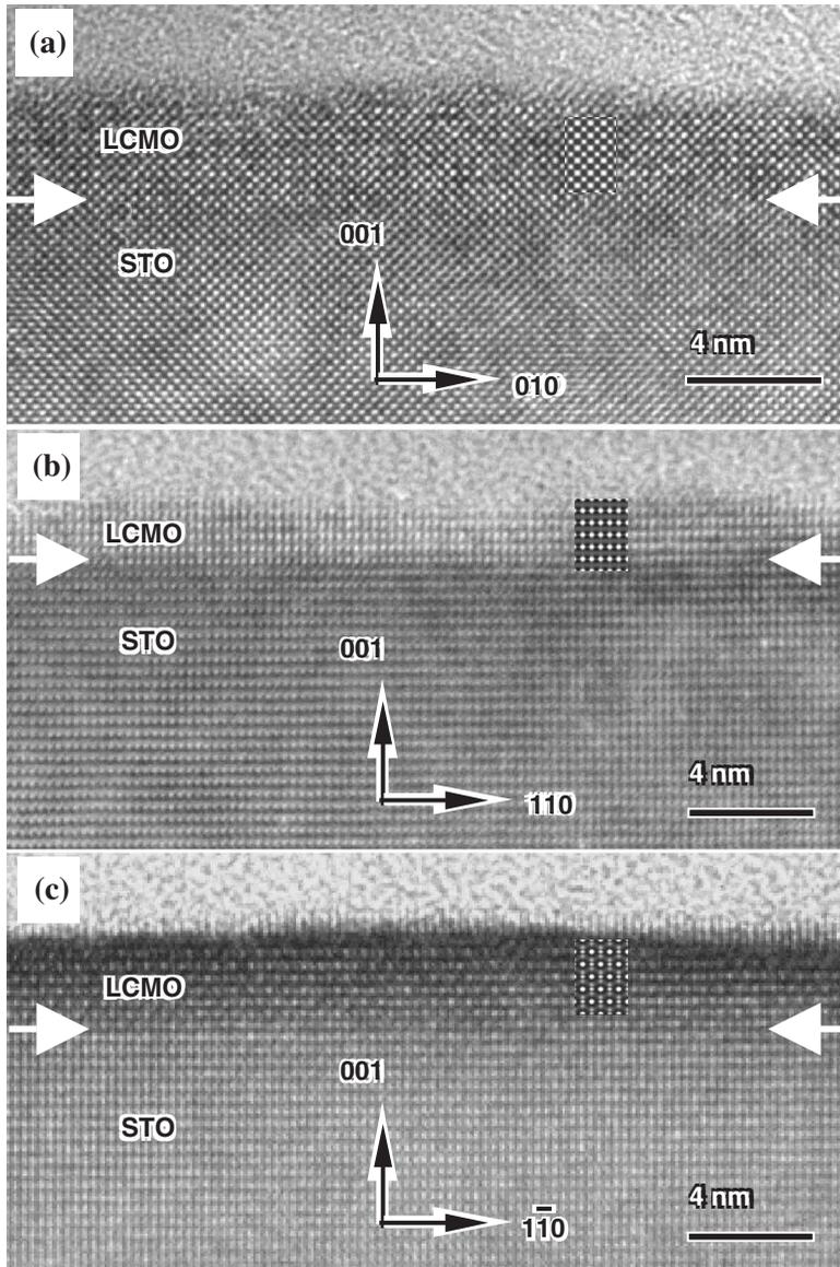
Figure 1. Cross-sectional HRTEM images of a 3 nm LCMO ultrathin film taken along (a)  $[100]_{\text{STO}}$ , (b)  $[110]_{\text{STO}}$  and (c)  $[110]_{\text{STO}}$  directions, respectively. Note the superstructure pattern in (c) is not presented in (b). The calculated images are given as insets: thickness  $t = 8$  nm and defocus value  $\Delta f = -45$  nm for (a), and  $-15$  nm for (b) and (c).
