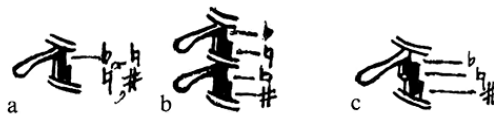
Figure 5 a. Hochbrucker single action b. Cousineau double-pedal single action c. Erard single pedal double action
