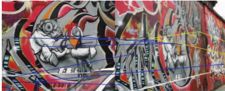
Figure 3.3: Matches (blue lines), between images after an affine viewpoint change, found by using the SIFT (OpenCV) salient point approach.
