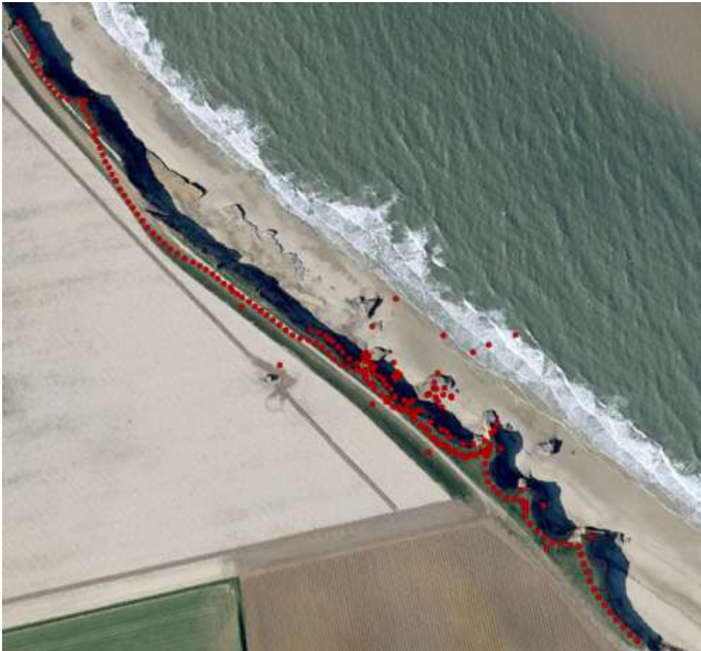
Figure 12 - 2011 Measured points along the coastline, mapping cliff bottom and top.
