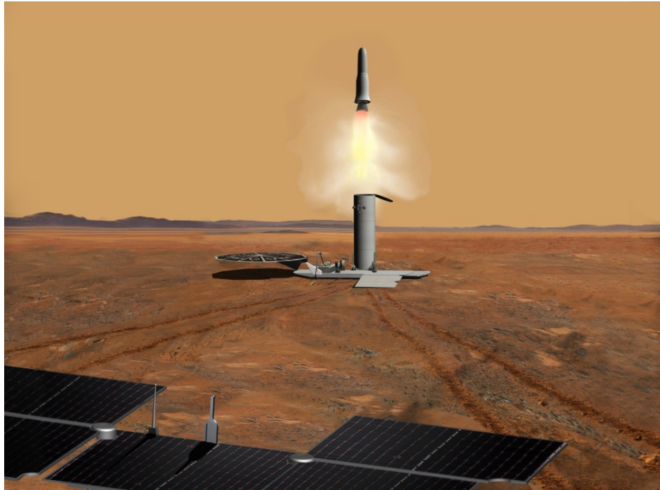
Figure 6. Artist's concept of the Mars Sample Return mission showing the ascent phase from the martian surface. Once the sample container reaches Mars orbit it will rendezvous with a Mars Sample Return Orbiter that returns the collected samples to Earth. Image Credit: Jet Propulsion Laboratory
