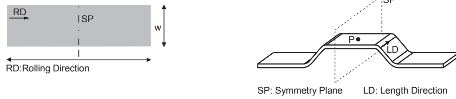
Figure 6.14: Friction experiment; Left: Specimen of the experiment; Right: Shape of the specimen after the forming operation.
