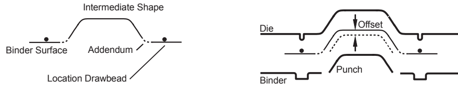
Figure 3.9: Example; Left: Illustration of a stamping operation based on the intermediate shape; Right: Derivation of the tool surfaces.
