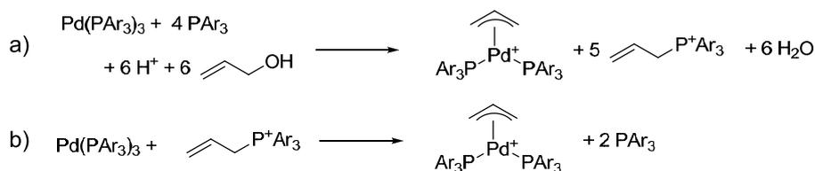
**Scheme 1.12.** Allylation of free phosphine with consumption of acid to form allyl phosphonium salts and water in the presence of a Pd(0) complex and b) the reverse reaction.<sup>78</sup>
