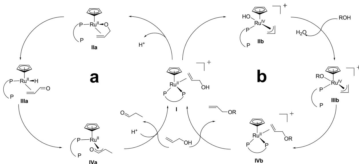
**Scheme 1.16.** Proposed mechanism of the catalytic a) isomerization and b) allylation of allyl alcohol by a ruthenium complex.<sup>82</sup>
