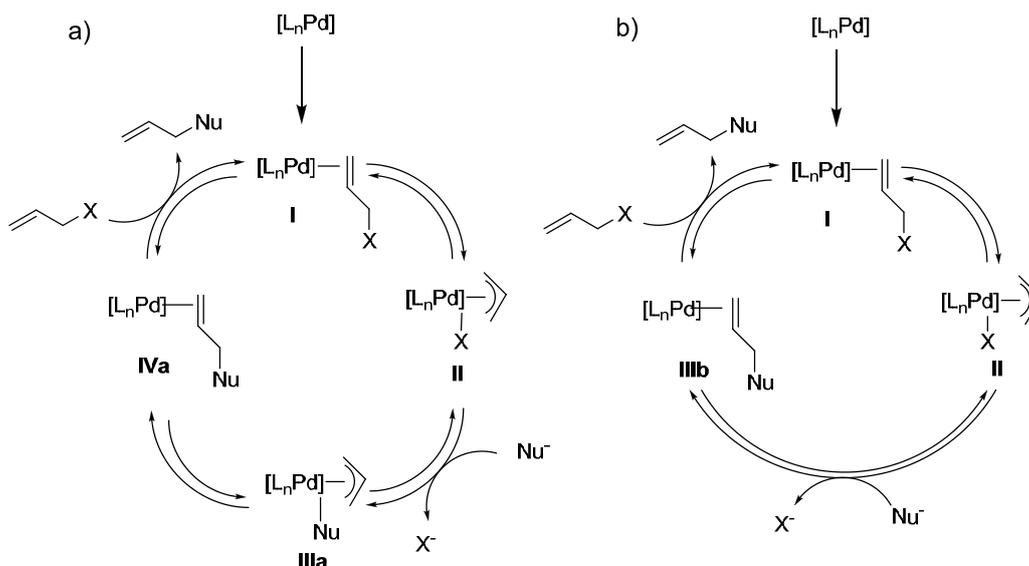
**Scheme 1.6.** Proposed mechanism for the Tsuji-Trost type allylation reactions of a) hard nucleophiles and b) soft nucleophiles.<sup>25</sup>
