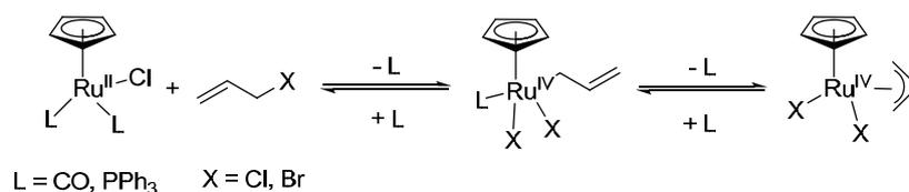
**Scheme 1.9.** Proposed intermediates in the oxidative addition of allyl-X onto RuCp(L<sub>2</sub>)X.<sup>52</sup>
