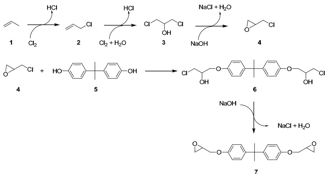
**Scheme 1.2.** Current process towards bisphenyl A diglycidyl ether.
