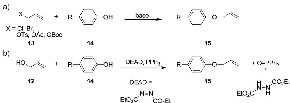
Scheme 1.5. Non-catalytic synthetic routes to allyl phenyl ethers.
