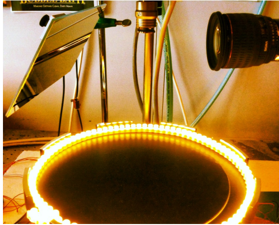
Figure 3.11 – The camera (right) and mirror (left) placement above the tilt platform where the LED light strip lights the dish (not shown) from below. The lights are placed at a slight angle underneath the place where the foam packing will ultimately sit. The leveling platform is black to enhance contrast. Due to the tilt of the mirror over the dish and the alignment of the camera the images are skewed and will be corrected.
