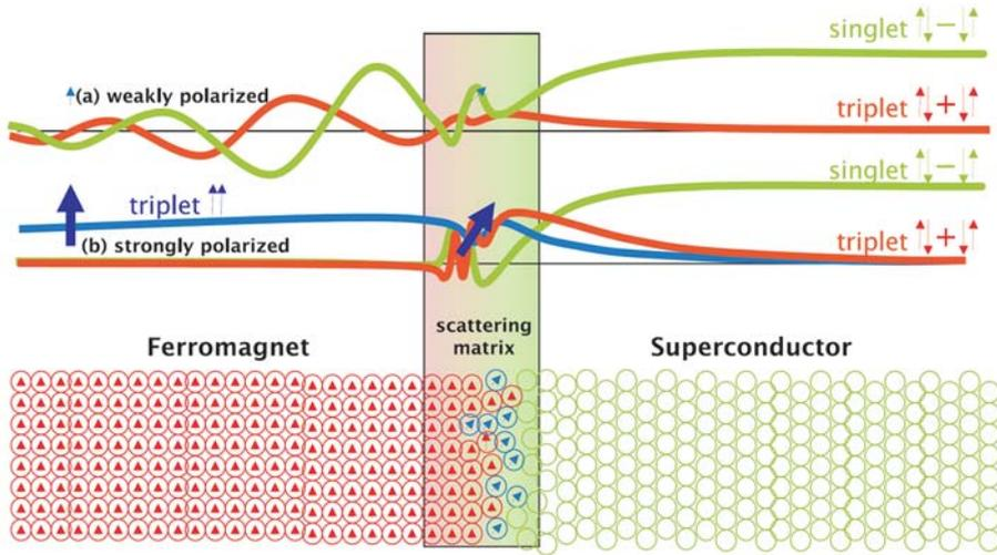
Figure 2.8: Calculation of the triplet components generated at a spin-active S/F interface, as taken from Eschrig *et al.* [40]. Top: weakly polarized ferromagnet, Bottom: strongly polarized ferromagnet
