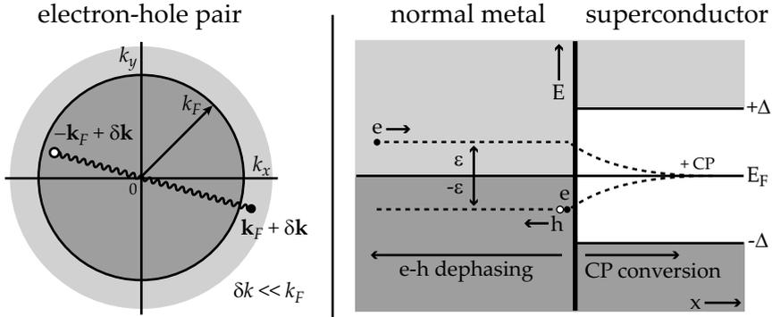
Figure 2.7: The right panel shows the Andreev reflection at a normal metal - superconductor interface. Upon reaching the interface, the incoming electron at energy  $\epsilon$  causes a hole reflection at energy  $-\epsilon$  (together they form the correlated electron-hole pair). The incoming electron itself and the missing electron in the valence band have entered the superconductor where they are converted into a Cooper pair. The left panel shows the correlated electron-hole in  $k$ -space.
