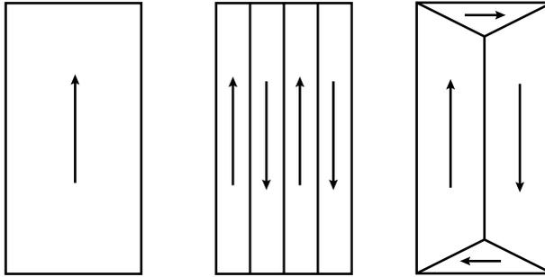
Figure 2.4: Different possible domain configurations in a ferromagnet, with from left to right a decrease of the induced field outside the ferromagnet.
