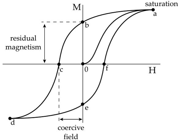
Figure 2.6: Hysteresis curve showing saturation magnetization (points a and d) remanent magnetization (points b and e) and coercive fields (points c and f).
