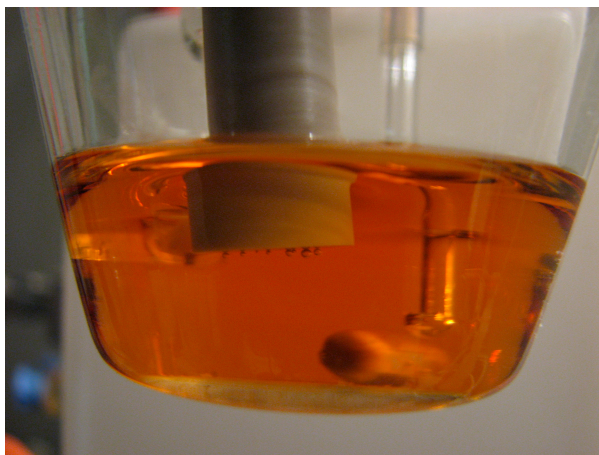
Fig. 3.9. Dihydrogen bubbles formed on the surface of the glassy carbon working electrode during the electrocatalysis of 0.5 mM [Ni(pbss)Fe(C 5 H 5 )(CO)]PF 6 in the presence of acetic acid. Object at the bottom of the cell is a stir-bar; the Pt wire counter electrode and the Ag/AgCl reference electrode are behind the working electrode.
