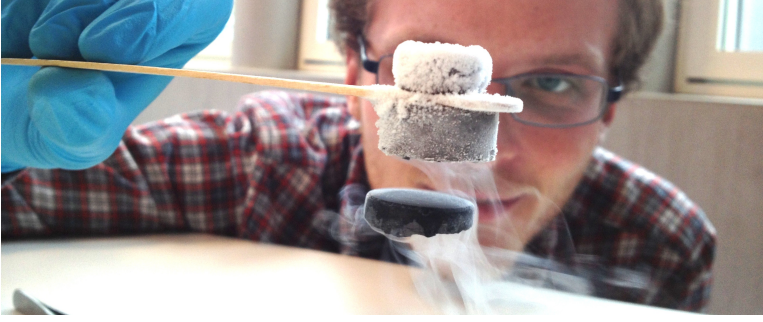
Figure 1.3: The high temperature superconductors are ill understood strongly correlated materials, and they are a prime example of quantum matter. Here the author is shown levitating a piece of superconducting YBCO at the Twente University.
